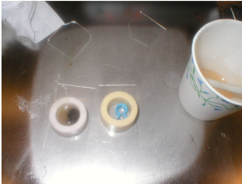
Image 2: Making epoxy mount
