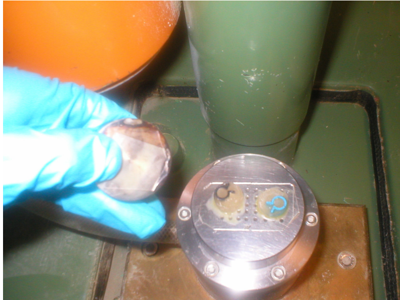
Image 3: Two glass slide mount holders fit on the grinding machine while one fits on the polishing metal cylinder
